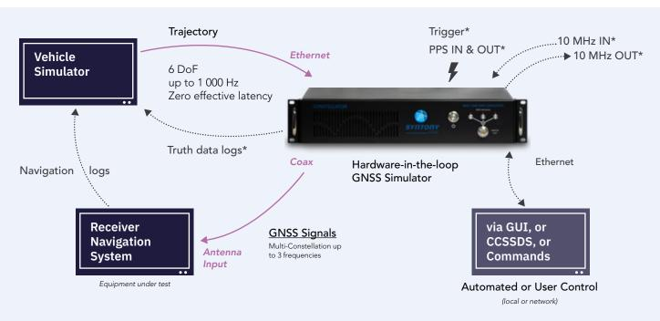
\*available by default on all Constellator™ units but not required for a hardware-in-the-loop test
