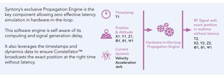
Constellator™'s hardware-in-the-loop is therefore plug and play as it will always ensure the GNSS signals are exactly on time and generate the exact trajectory described in input.
