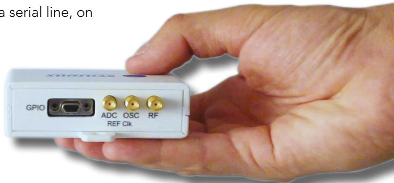
« GNSS Handheld recorder » is currently embedded on UAVs for reflectrometry applications by some German and French Universities
